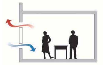
Single sided ventilation – via opening window, drawing air in by natural convection currents. This air will typically mix with warm air rising from radiators, etc.
