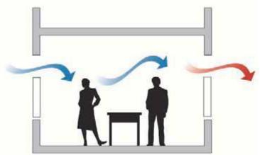
Cross Ventilation, could also draw fresh air from a central corridor or atrium. See Mechanical Supply Only below.
