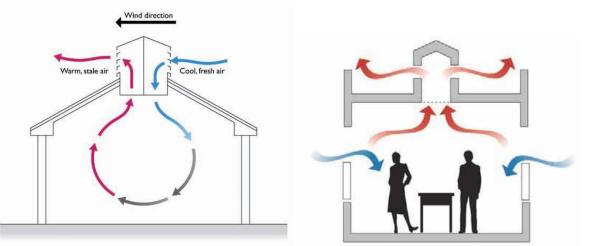
Passive Ventilation, such as "Windcatcher" on the left and "Stack" effect on the right, use a combination of natural convection and wind speed to draw fresh air in. They can also incorporate supply fans, to supplement supply air when wind direction or strength fluctuates and typically include external weather sensing, and automated controls. "As Installed Records" and Service Records should be reviewed to identify the type of system in use
